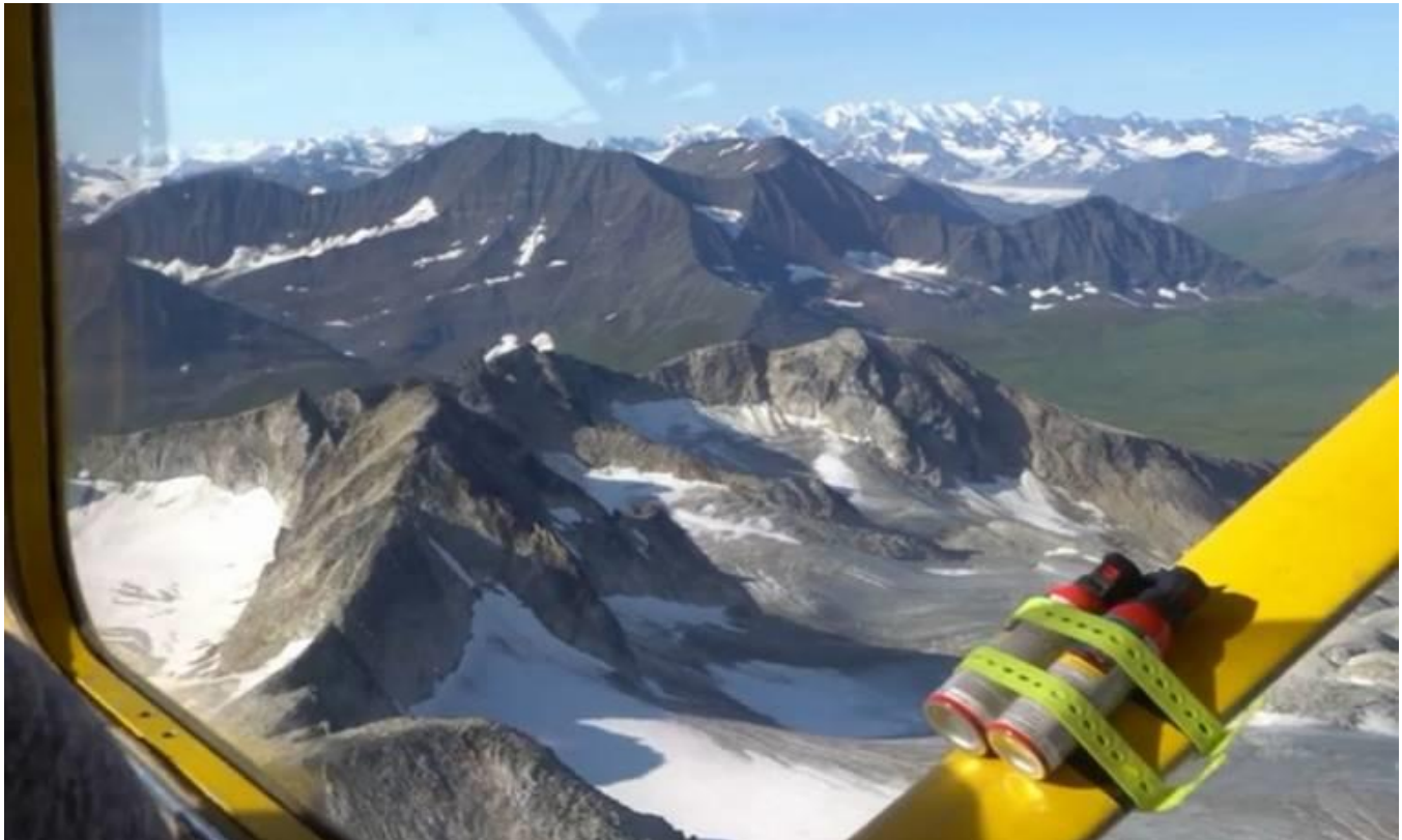
How to safely transport bear spray in a fixed-wing aircraft on wheels without an external storage compartment.
